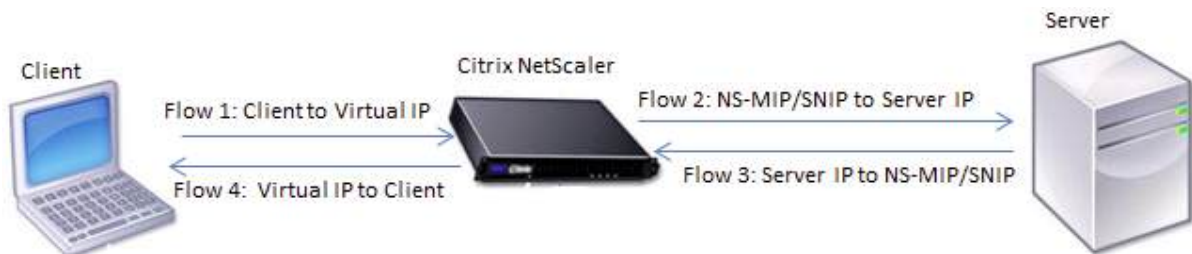
Figure 1. Citrix ADC Flow Sequence
