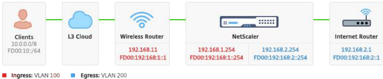
Figure: A simple depiction of a Gi-LAN
